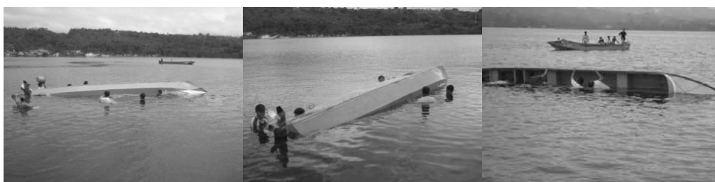
Fig. 4. A floating test for capsized condition.
