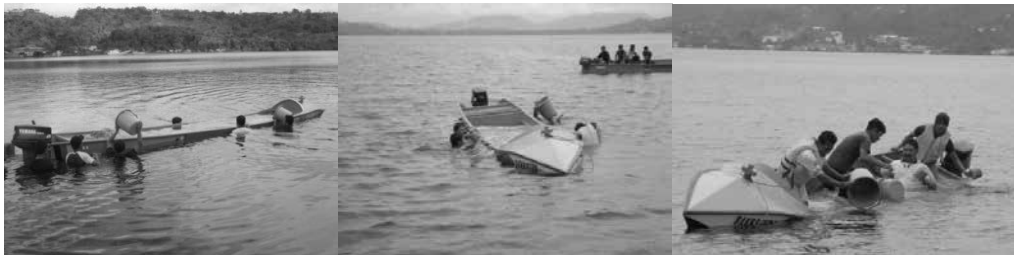
Fig. 3. A floating test for upright position.
