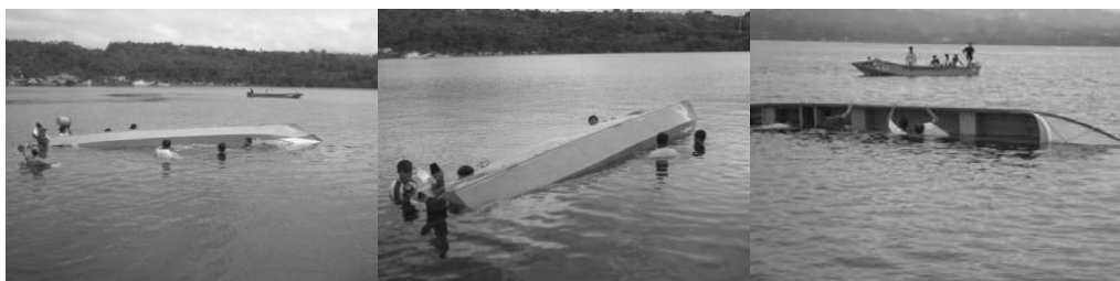
Fig. 4. A floating test for capsized condition.
